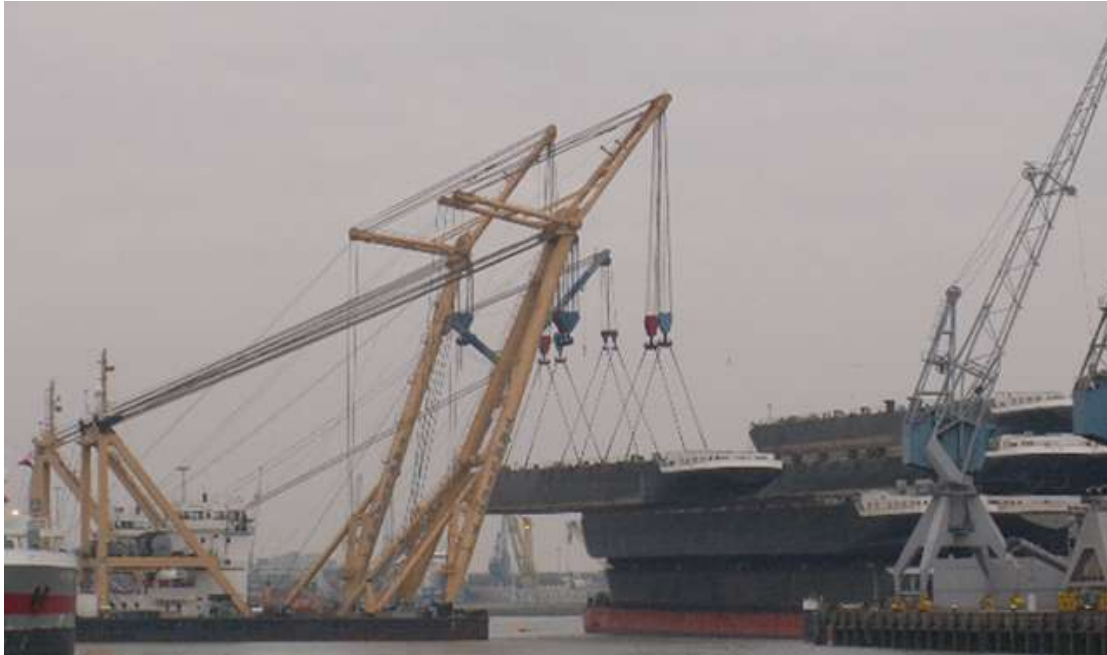
The Taklift 6 and 7 (together with a Matador sheerleg) seen unloading casco's from the Sainty barge at the Waalhaven Rotterdam.
