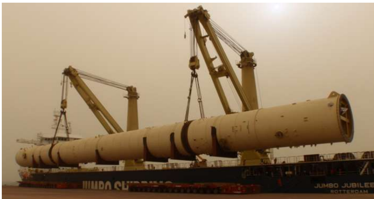
Above seen Mammoet - Saudi Arabia receiving a 1431 ton - 110 meter column from the Jumbo Jubilee in Jubail Industrial Port - Saudi Arabia on 4th March Below seen a photo of the 15 km transport to NCP Project in Jubail Industrial City. Column was safely delivered on 12th March
