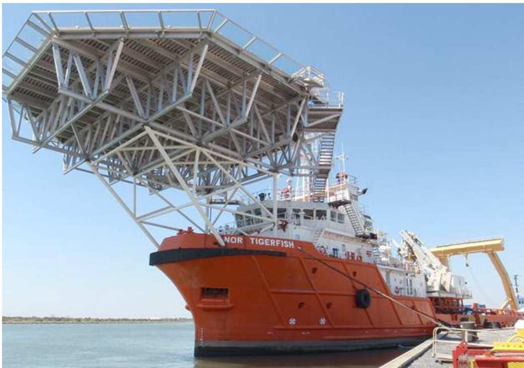
Nor Tigerfish seen at the Bollinger yard in Port Fourchon (USA) with the new installed helideck Photo : NOR Offshore (c)
