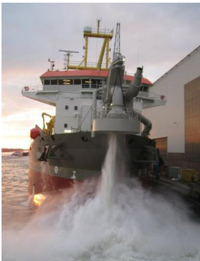
The brandnew TSHD GATEWAY seen testing her pumps prior her yard trials Photo : Jan Gossen Roos ©
