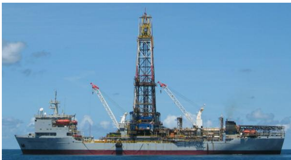
Above seen the Noble Muravlenko , a Pelican class dynamically positioned drillship working offshore Brasil in Campos Basin. The rig is under contract of Petrobras - Photo : Capt. Dirk Struijf ©
