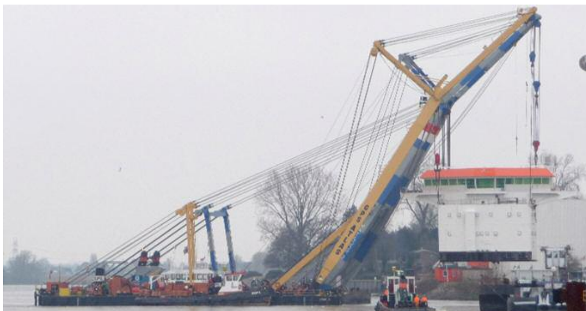
The sheerlegs GPS ATLAS and MATADOR 2 seen lifting the new superstructure for the recently launched TSHD WILLEM VAN ORANJE at the IHC-Merwede shipyard Photo : Jan Oosterboer ©
