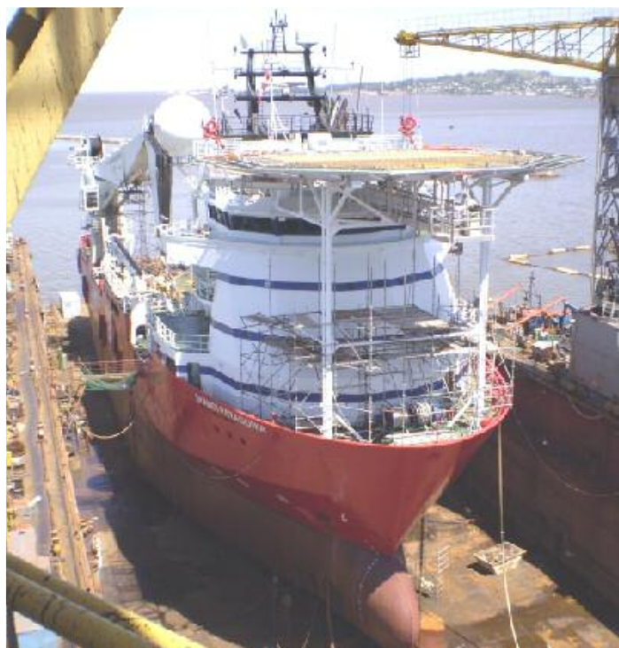
Above seen the 13,920 HP Multi-Functional Support Vessel SKANDI PATAGONIA (built 2000) undergoing Special Survey at Tsakos' Montevideo (Uruguay) floating dock. This vessel was completed to Total's specifications for their Tierra del Fuego production area.
