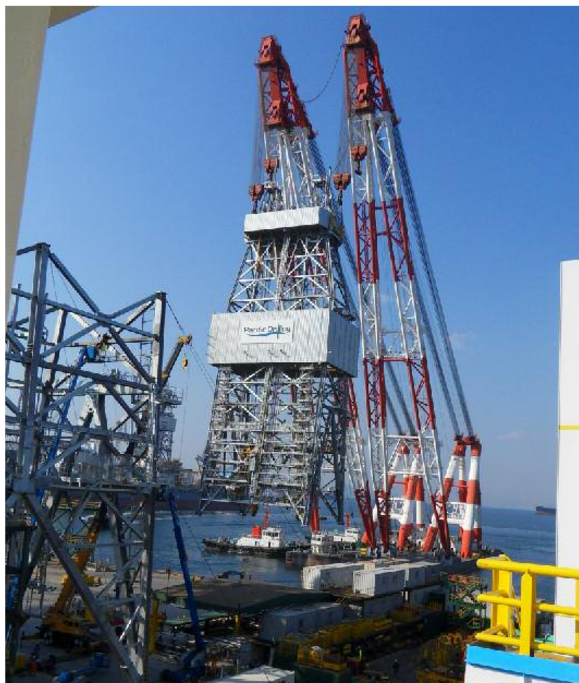
Derrick being lifted from quayside then onto Ultra deepwater Drill ship Pacific Bora at Samsung Heavy Industries Korea
