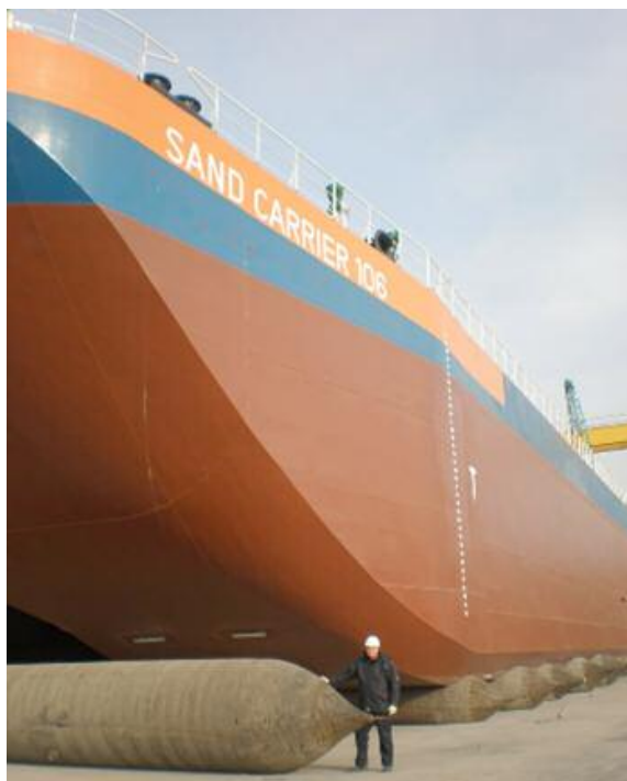
Van Oord's SAND CARRIER 106 ( 5th barge out a series of 6) seen ready for launching at Dalian Shipyard in China, after the launch the DMS KINGFISHER will tow the barge to Batam (Indonesia)
