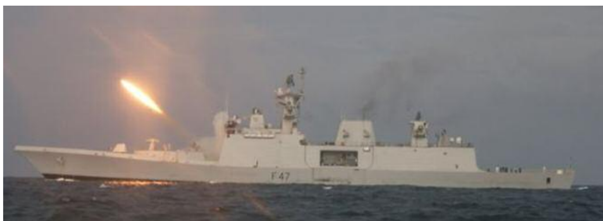
The Shivalik undergoing weapons trials on 25 September 2009. She is seen here firing a 90R missile from her RBU-6000 launcher.
