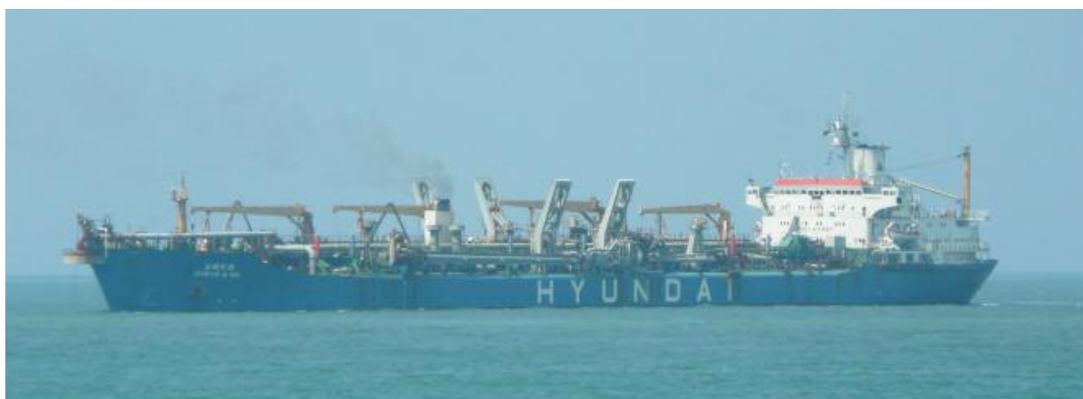
The Korean dredger GORYO – 6HO seen operating off Colombo Port, the dredger was originally built in 1985 as bulk carrier and was converted to sand carrier / dredger in 2001. The Goryo-6HO can carry up to 27,000m3 of material.
