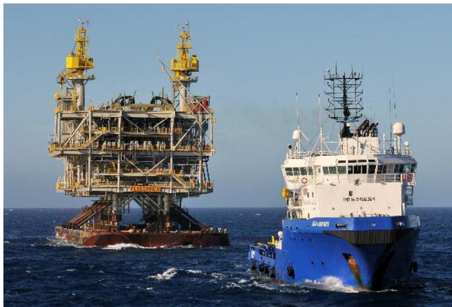
The Sea Leopard seen towing the barge H-406 loaded with the Peregrino-B topside approaching Heerema's HERMOD in Brazilian waters
