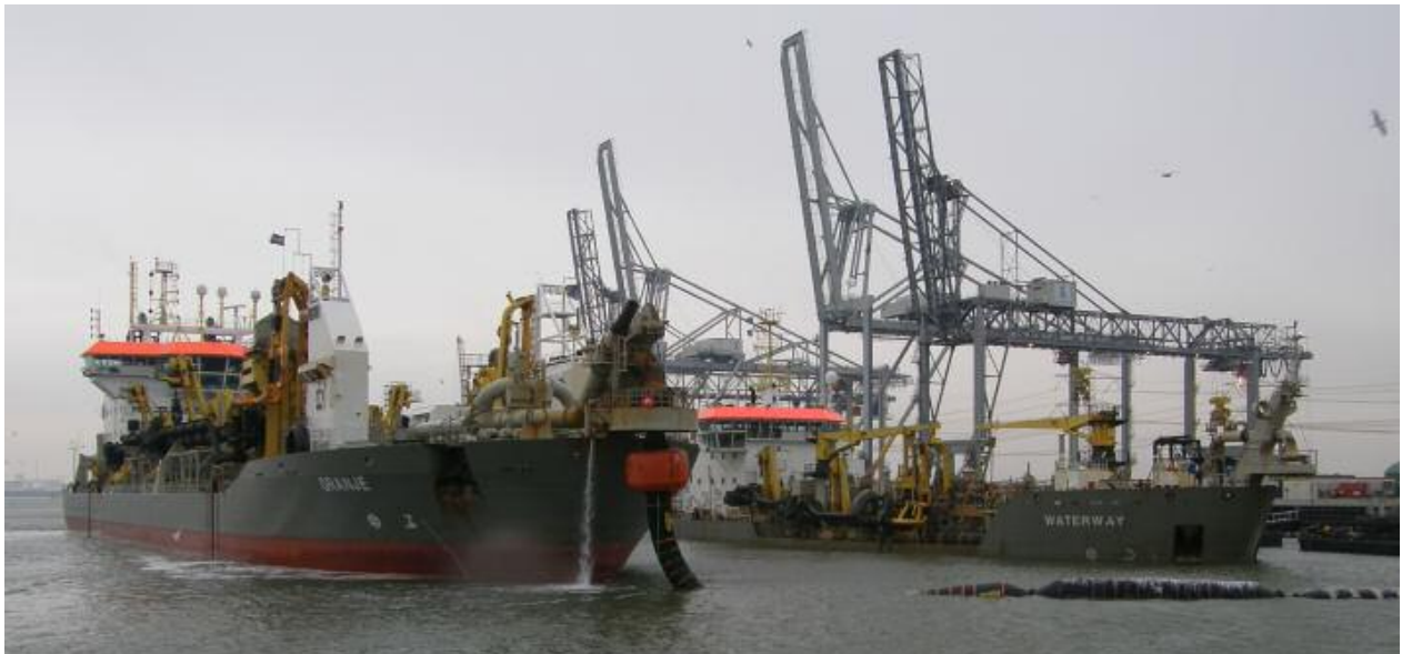
Above seen the TSHD Oranje and the TSHD Waterway operating close to each other in the Mississippi Harbour in Rotterdam-Europoort , The Waterway is pumping "dirty" slib towards the Slufter and the Oranje is pumping sand towards Oostvoorne to increase the strength of the beach
