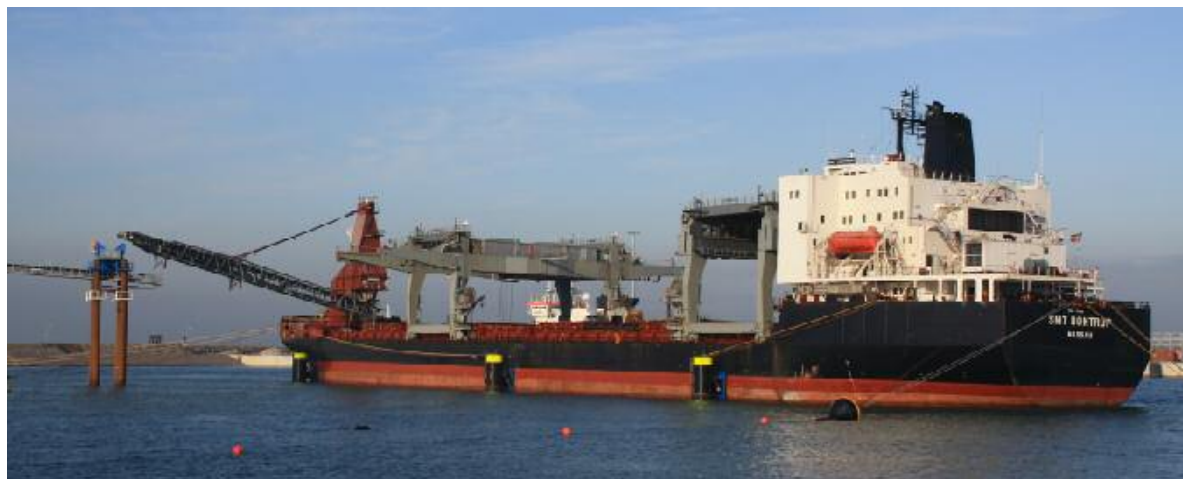
The SMT BONTRUP seen discharging rocks / stones for the Maasvlakte 2 project , in total will 5 million tons rock/stones will be delivered
