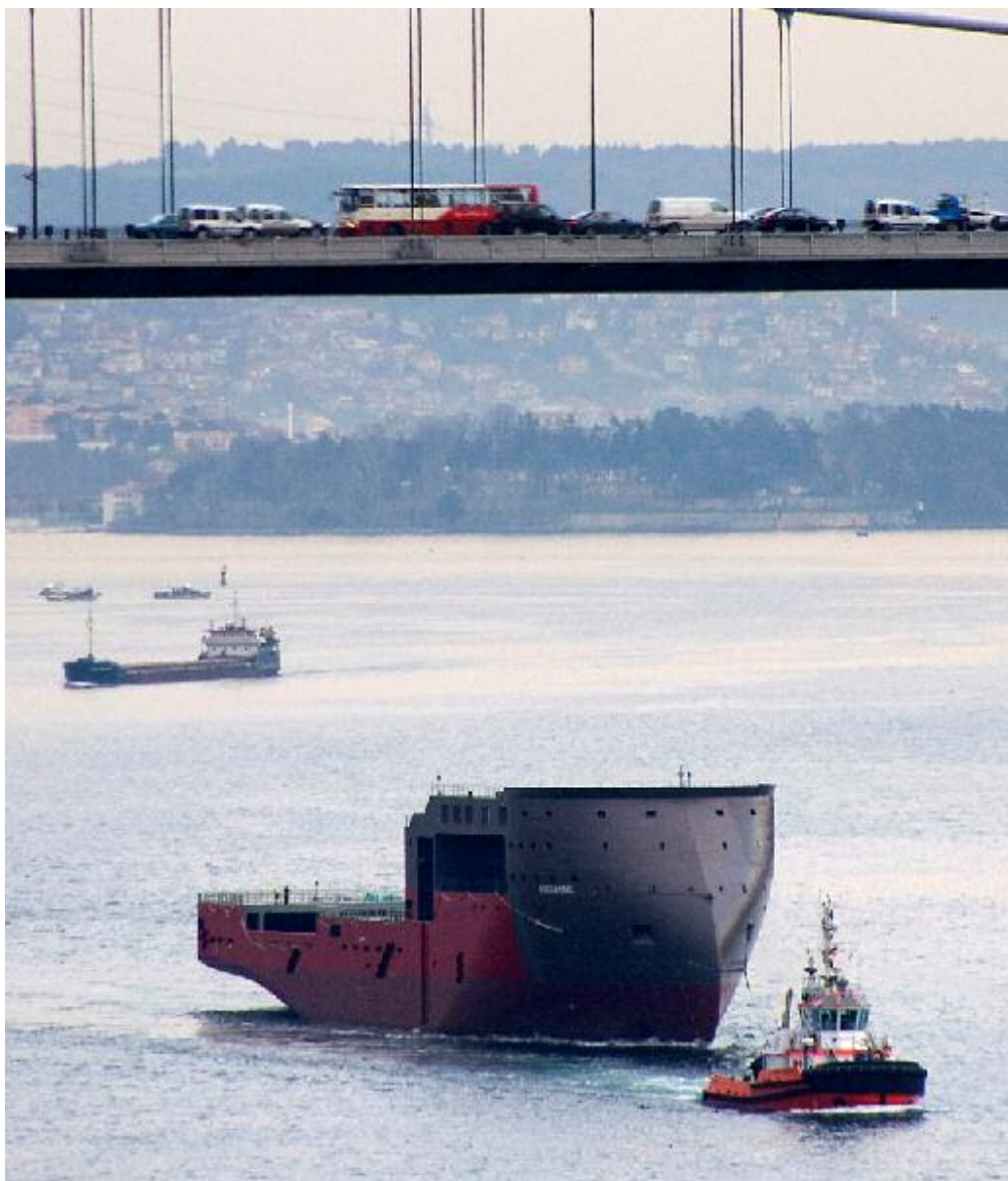
Above seen the Stadt Valiant passing the Bosphorus on its maiden voyage, towing the hull " Karianne " from Kerch, Ukraine to Ulstein Verft in Ulsteinvik, Norway. ETA Ulsteinvik is at the end of January. Stadt Valiant is a new building of Stadt Sjøtransport AS , and with 90 tonnes BP (87 tonnes cont) it will be one of the most powerful tugs of this size in Norway. Photos : Ekrem Şerif Egeli ©
