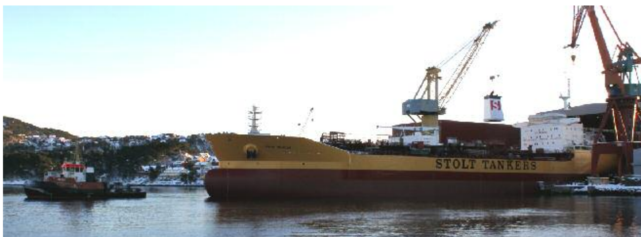
Above and below seen the tug WOLF towing the new building STOLT BRELAND out of the drydock on the STX shipyard in Florø, Norway. WOLF is a Bugsier tug on bareboat contract to Stadt Sjøtransport AS. It has two Voith propellers and BP 46 tonnes. Photo's : Egil Knutsen ©
