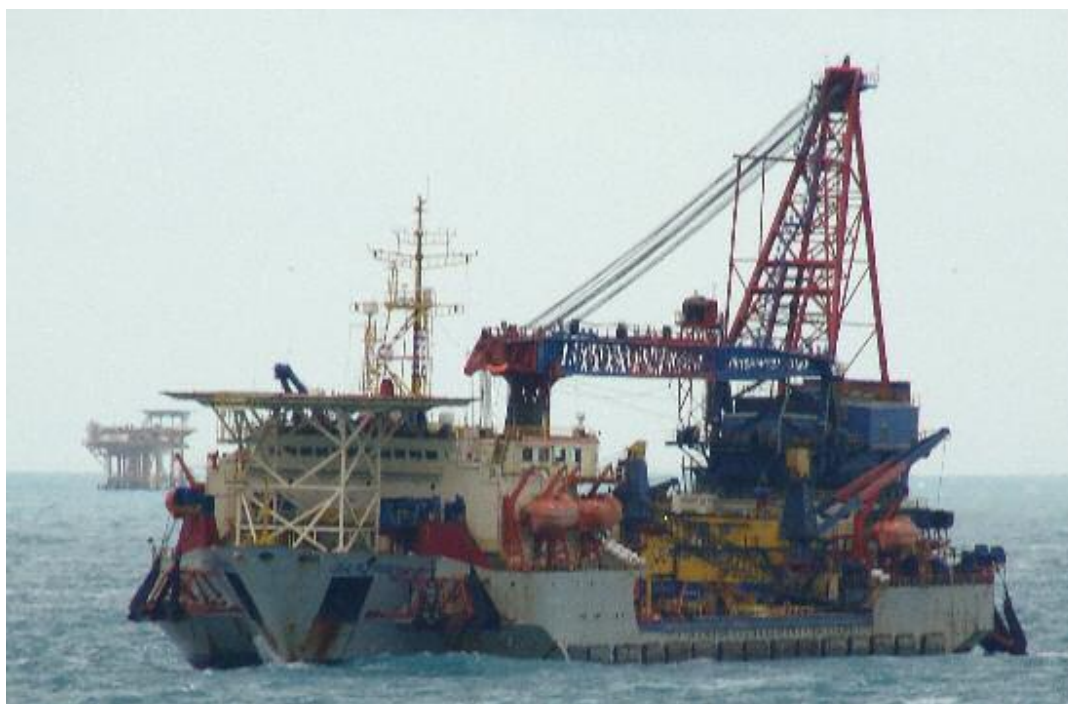
The converted drillship, now crane vessel GARZPROM 1 (ex Gazprom 1) seen in the Bay of Campeche (Mexico), riding out some swell and gales.
