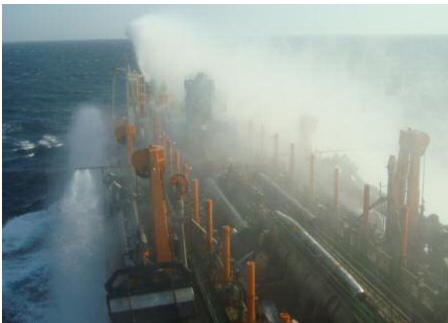
Above seen a Dutch TSHD testing her anti piracy equipment , equipped with razor wire and powerful water spray system - Photo : Crew TSHD © (For safety reasons for the crew and vessel no name of the vessel mentioned)
