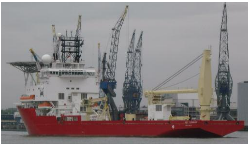
The IHC-DE MERWEDE built HOS ACHIEVER departed from the Wiltonharbour after installation of the new HUISMAN crane Photo : Jan Simons ©
