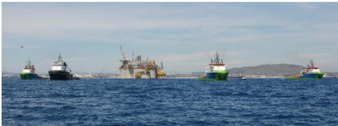
1 POSH-SEMCO and 3 FAIRMOUNT tugs departed with the Adriatic LNG terminal from La Linea (Spain) with destination Venice (Italy)
