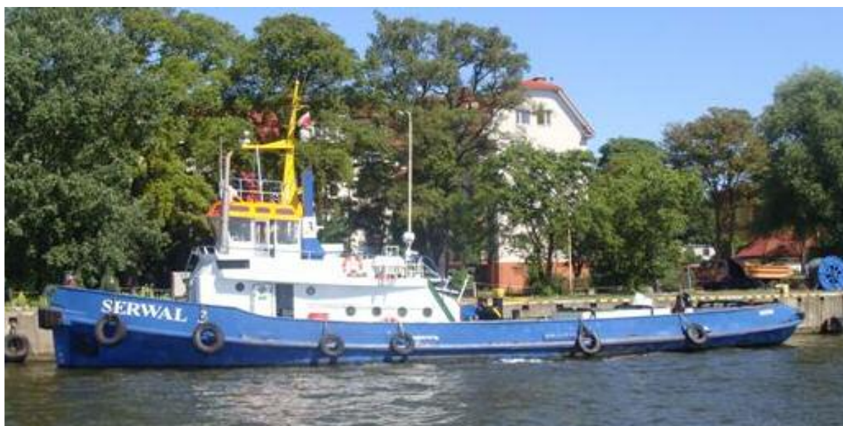
The 1962 built 29 mtr SERWAL-3 is the former MULTRATUG 14 and built as the PETRONELLA J.GOEDKOOP , the tug with an bollard pull of 18 ton is at present in charter by Porject Zegluga, Szczecin, Polen.
