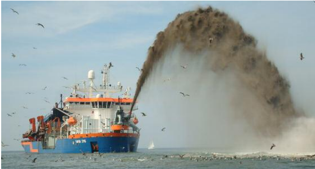
The HAM 316 seen rainbowing of the Dutch coast Photo : Captain & Ch.Eng MOB boat ©
