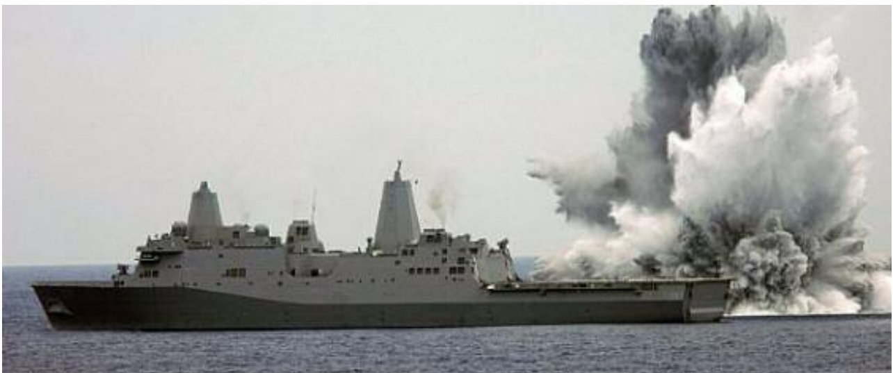
A 10,000-pound underwater explosion rocks the amphibious transport dock USS Mesa Verde (LPD 19) during a shock test off the Florida coast. The test is part of Navy trials for the San Antonio-class ship, which was commissioned last December. Photo : U.S. Navy
