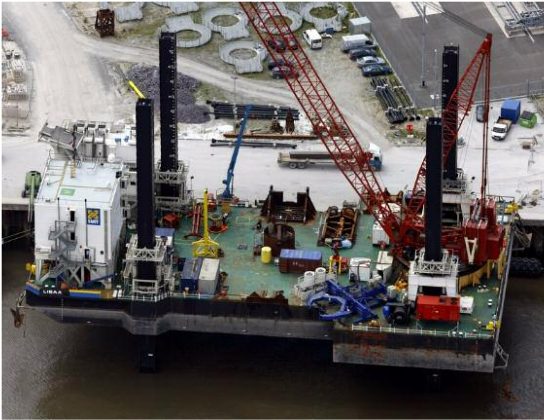
The SMIT operated jack-up work-platform LISA-A seen standing on her legs alongside in port Photo : Jonathan Webb - www.webbaviation.co.uk ©
