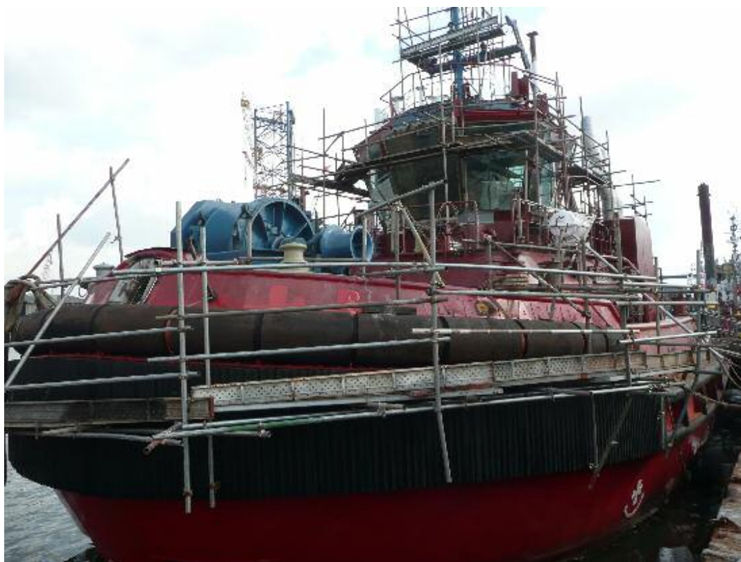
A Rotor tug 80 with yard number 820 seen under construction at the ASL yard in Singapore
