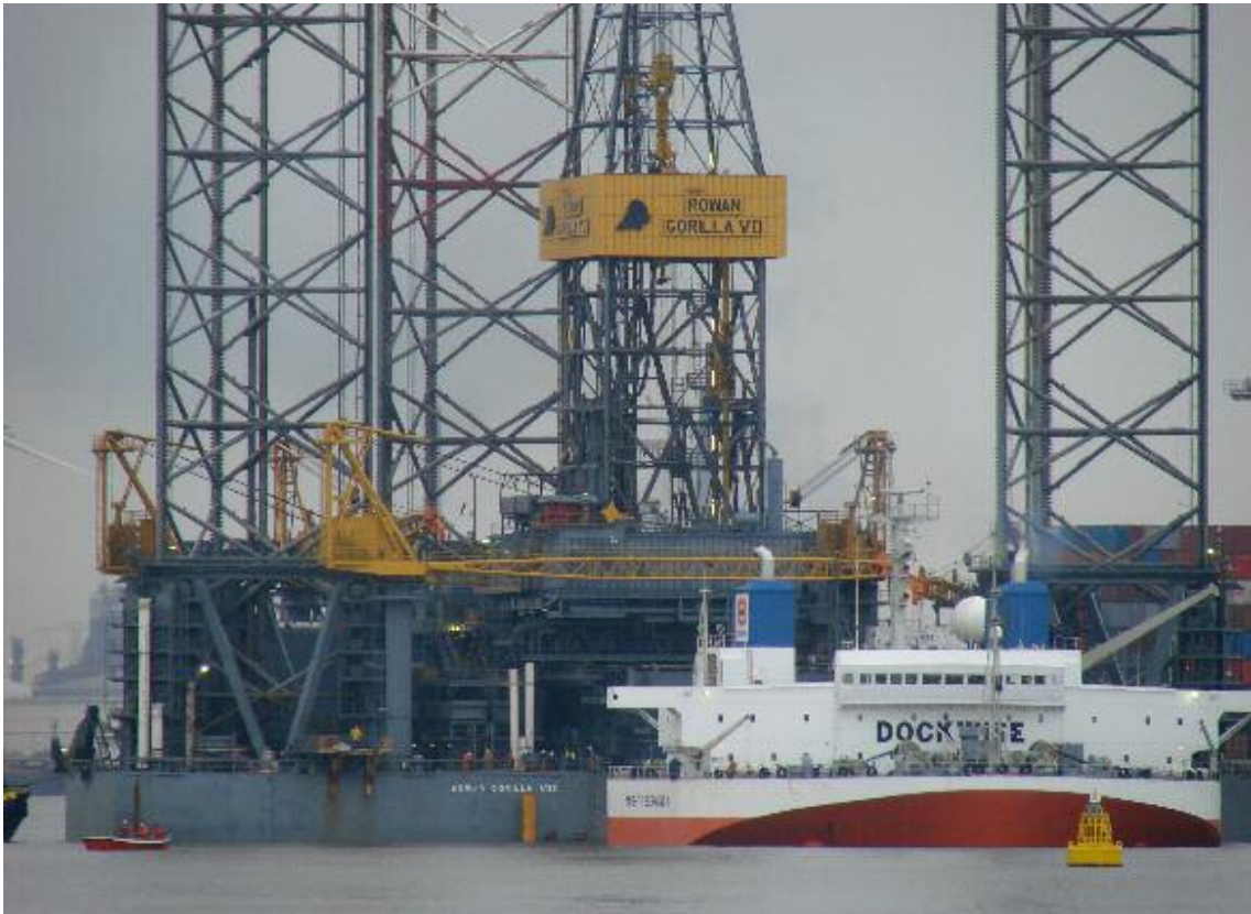
The MIGHTY SERVANT 1 seen submerged in Rotterdam-Europoort when loading the ROWAN GORILLA VII Photo : Frans Slob - Dockwise Shipping B.V. ©
