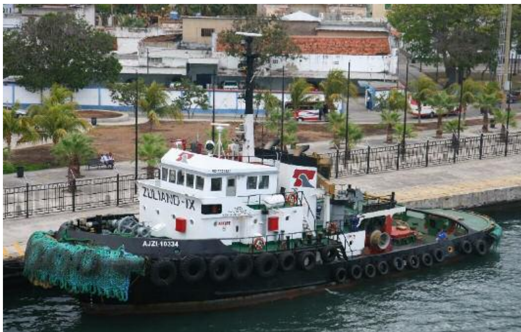
The 1979 built 33 mtr long and 3200 hp tug ZULIANO-IX (40 ton BP) seen in Puerto Cabello.
