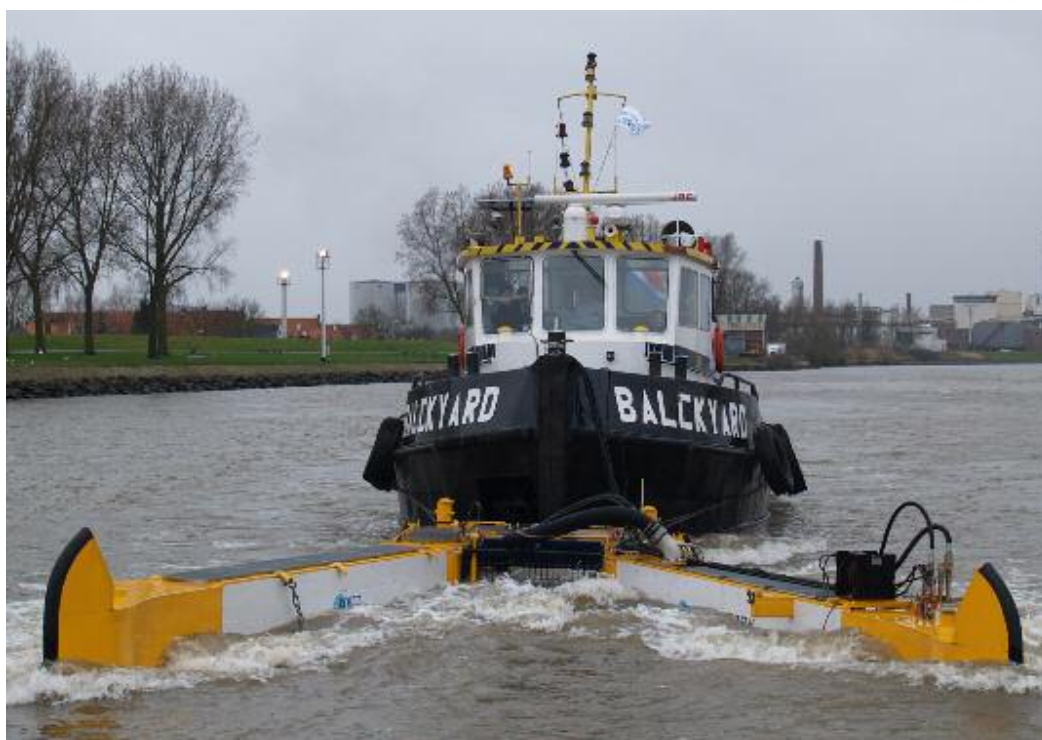
The BALCKYARD showing the KOSQ (Kampers Oil Spill Equipment) VICTORY oil sweeper.
