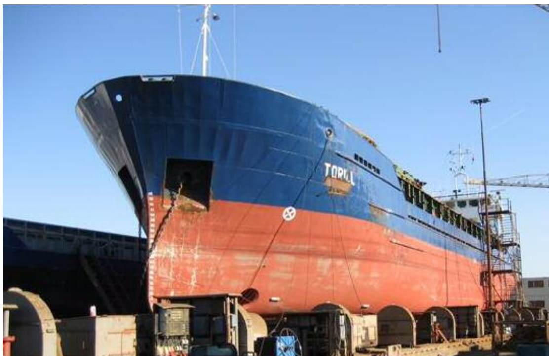
The mv Torill ( ex Arklow March / Fehn Trader) at Dockside Ship Facilities / former Bolnes Shipyard's slipway for class renewal.
