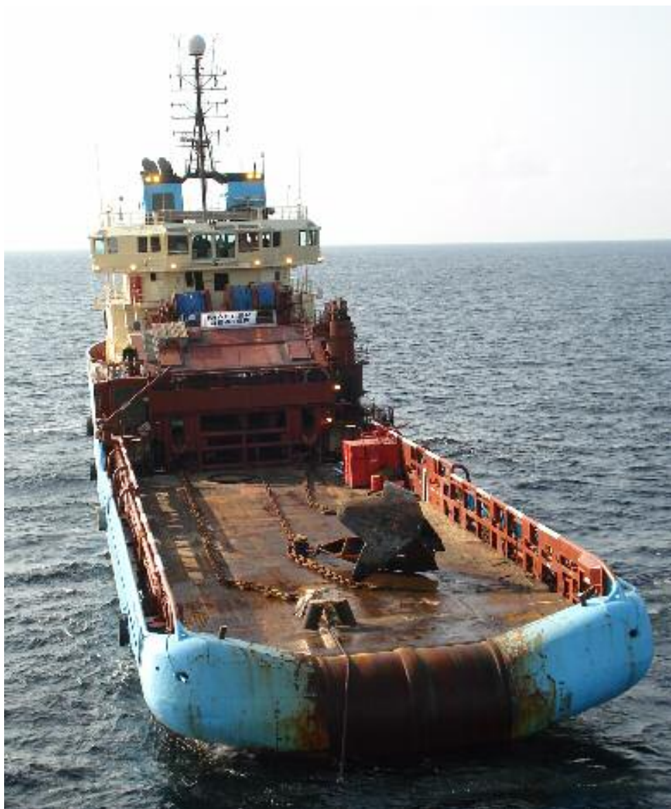
The AHTSV MAERSK BEATER doing anchor handling offshore Angola for the TRANSOCEAN rig MG HULME JR. Photo : Capt. Christian Schmidt ©
