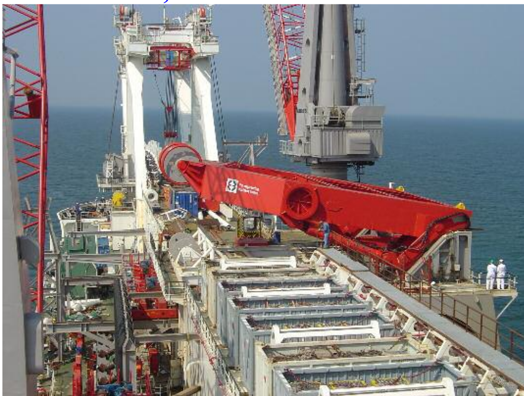
Testing of the PLET installation frame onboard pipe laying vessel Audacia off Kakinada.
