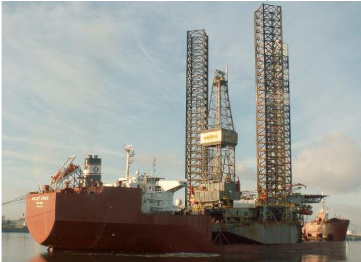
The ENSCO 85 was shifted from Keppel-Verolme shipyard to the Caland Canal where the rig was loaded onboard the WILLIFT EAGLE – Photo's : Jan Oosterboer ©
