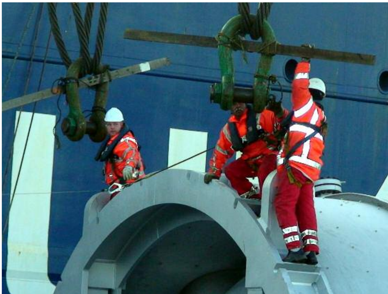
JUMBO crewmembers seen rigging the 1200 tons reactor prior loading onboard the FAIRPARTNER Photo : Richard L. Krabbendam ©
