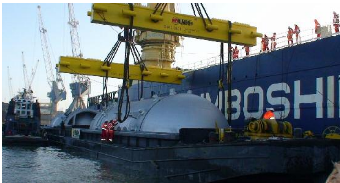
The FAIRPARTNER seen loading 2 pieces with a weight of 1200 tons reactors in Rotterdam
