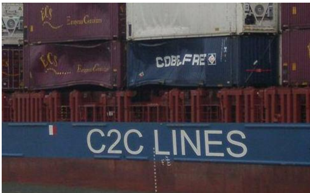
The C2C ASTRALIS enroute from Waterford to Zeebrugge encountered Westerly winds upto Force 11 Bft near Lands End which created damage to several containers and the gangway on starboard side of the vessel
