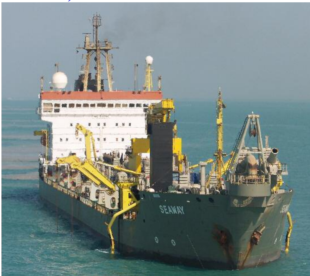
The TSHD SEAWAY seen dredging in the Outer Channel of Busher Port, Iran
