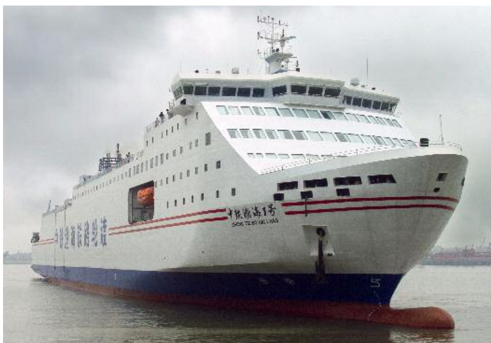
The Chinese ferry ZHONG TIE BO HAI 1 HAO is equipped with 4 x MAK 9 M 25 Engines
