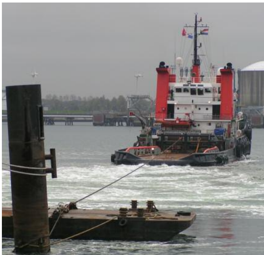
Heerema's HUSKY seen performing a bollard pull test in Rotterdam-Caland canal
