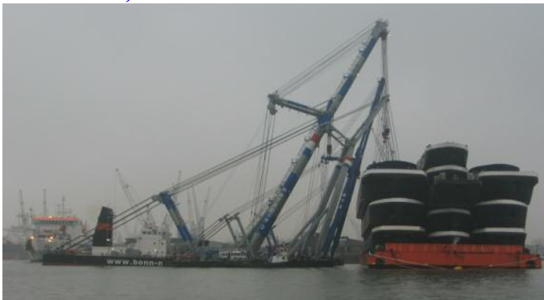
In the port of Rotterdam sheerlegs started with offloading the newbuilding hulls from the Sainty No 5 Photo : Jan Simons ©
