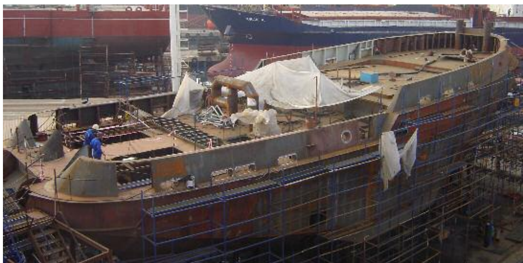
The hull of the TRITON , newbuilding 65 ton BP Rampart 3200 tug for ISKES tugs in IJmuiden, seen under construction at the Dearsan Yard in Tuzla (Turkey).
