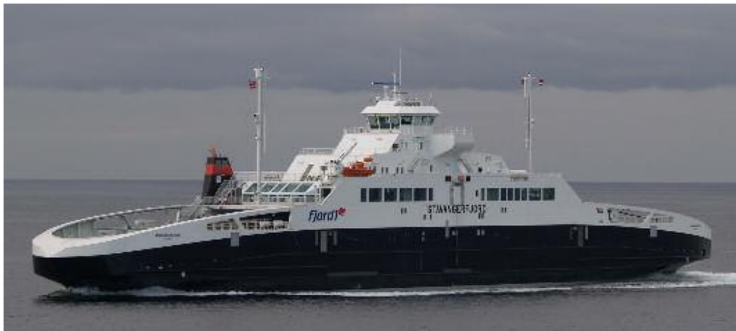
The ferry STAVANGERFJORD is using environmental friendly LNG propulsion
