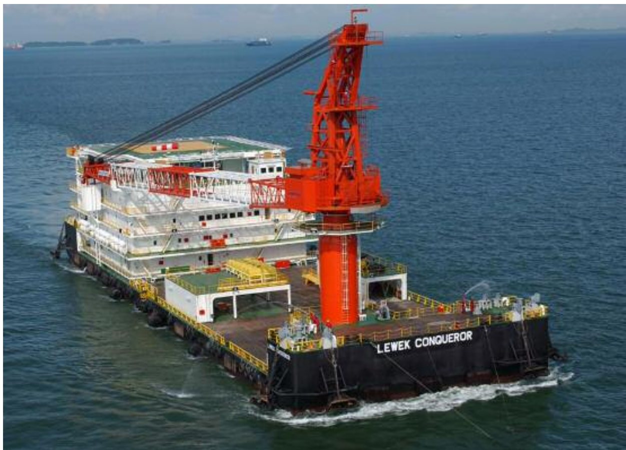
The 142 mtr accommodation/crane barge LEWEK CONQUEROR is built during 2004 at P.T. Nam Indah Mutiara Shipyard in Batam, Indonesia, Onboard is a Seatrax 350-ton kingpost pedestal crane with 210-ft boom is installed
