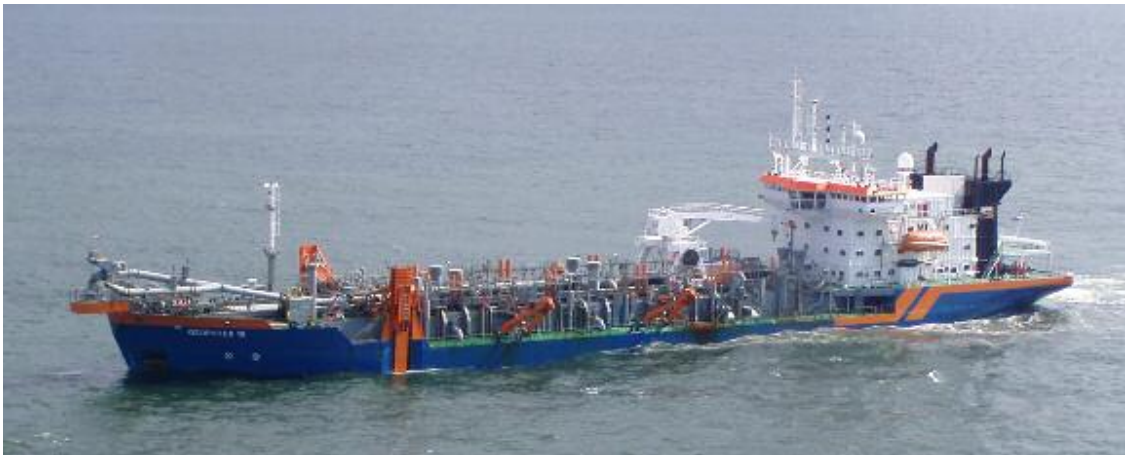
The GEOPOTES 15 seen operating near Den Helder where the dredger at present is dredging and transporting 7 million cub mtr of sand to improve the quality of the coast.
