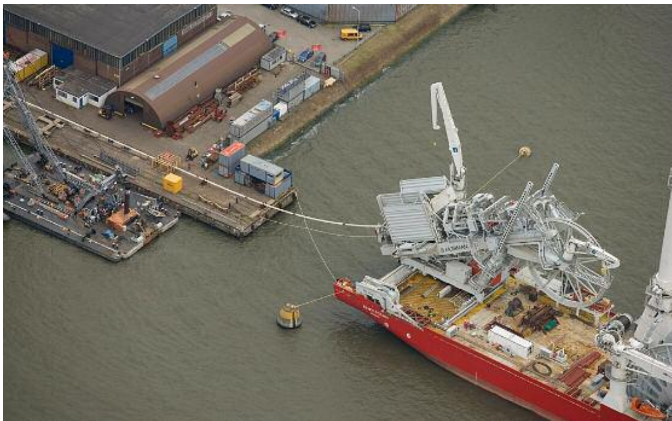
Photo Top : The ridged pipelay vessel SEVEN OCEANS seen from the sky as it is pulling the 850 metres long 12 inch test lay pipe from the quay at Sledge Hammer .
