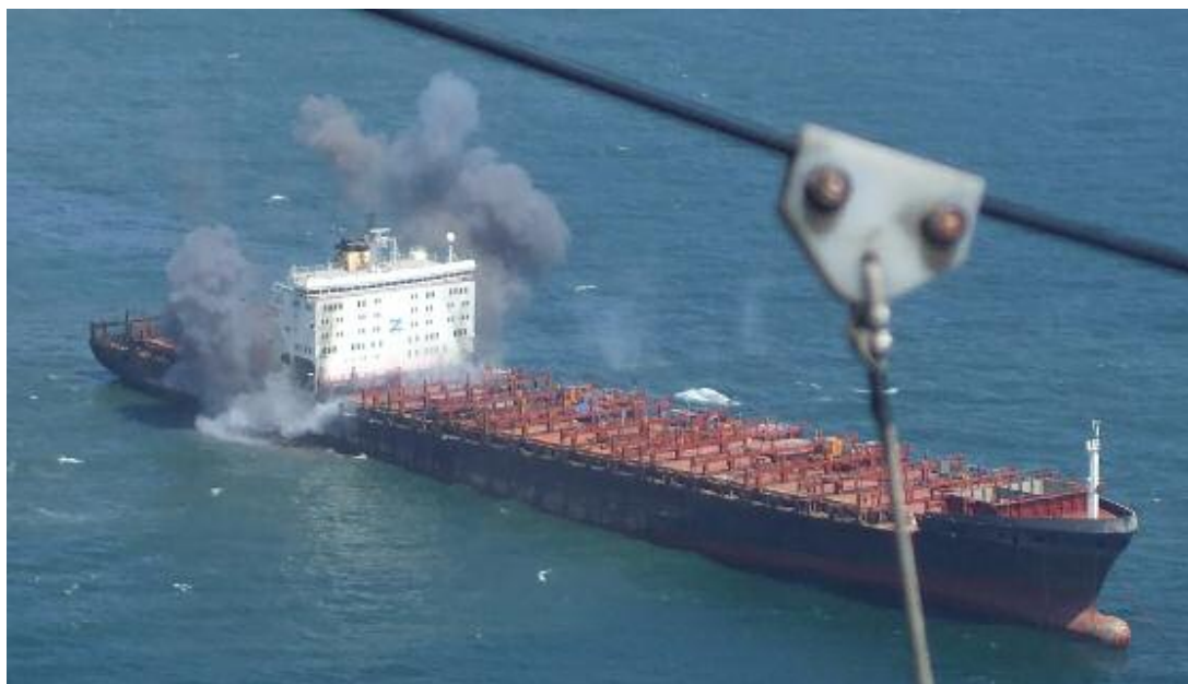
Top : Explosives are used in an attempt to split the deck plates as can be seen above.
