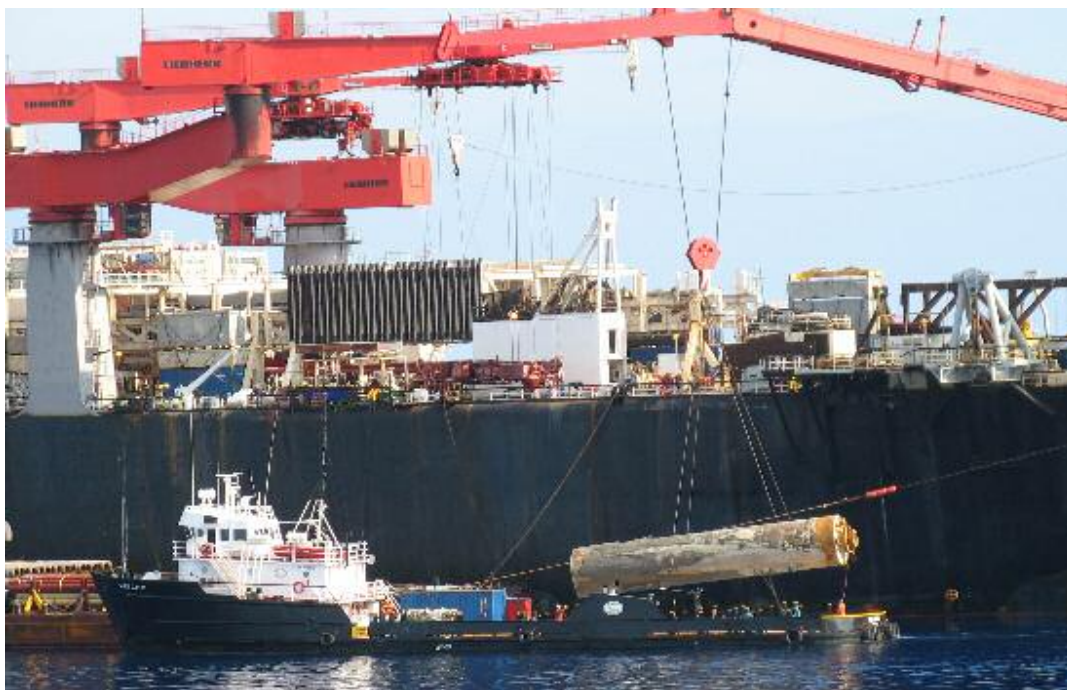
The Solitaire seen loading a suction pile on to the supply vessel Kurt David in the Gulf of Mexico.
