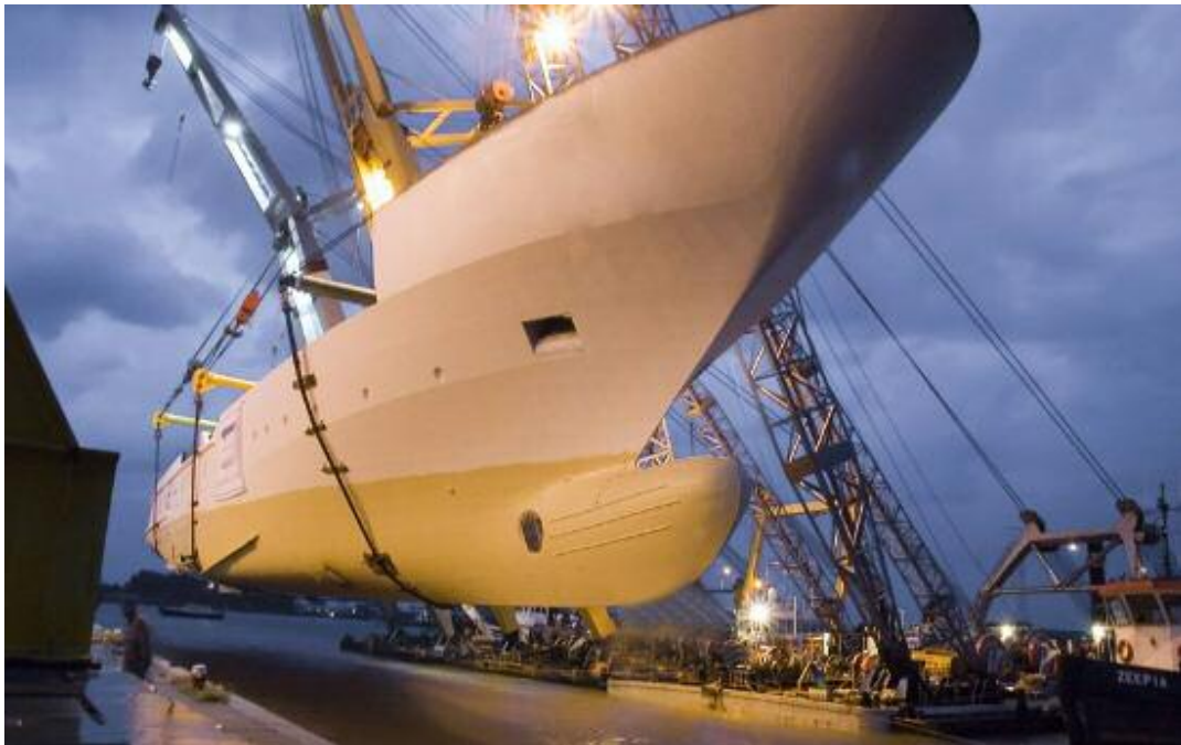
3 sheerlegs, GPS ATLAS , GPS AJAX and MATADOR were required to lift the above megayacht into the water at the Zwanenburg shipyard in Krimpen aan de IJssel Photo : GPS Marine services BV ©
