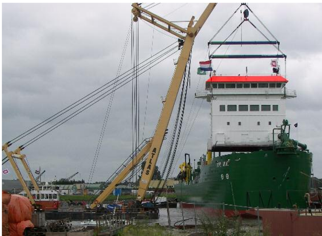
The sheerlegs GPS ATLAS seen installing the superstructure of the newbuilding trailing suction dredger TSHD ABUL at the IHC Slidrecht shipyard.
