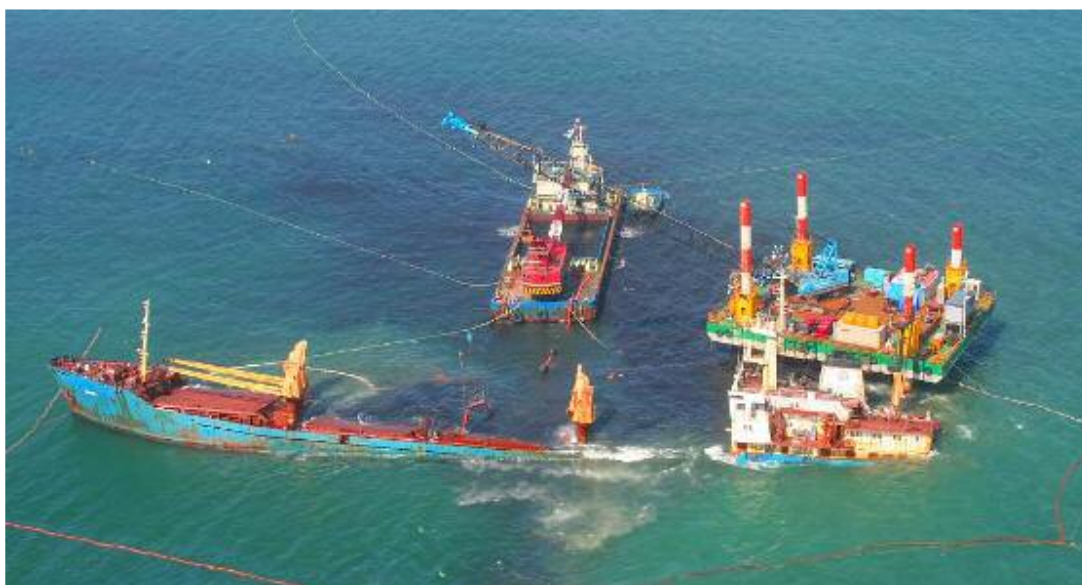
Above seen TITAN salvage working on the sunken JANE on the East Coast of Japan, near the port of Isohama, the 1987 built Jane sank after the engine room started flooding, and the master decided to ground the vessel before the engine stopped.
