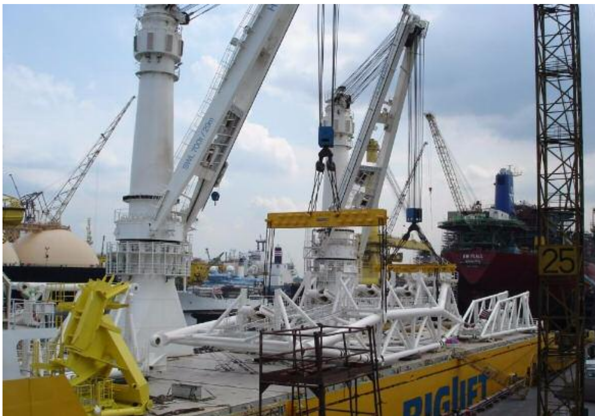
The HAPPY BUCCANEER seen at Sembawang shipyard in Singapore lifting off the Huisman built Stinger for the Pipe layer Heavy lift vessel Sapura 3000 Photo : Stephen Carson ©
