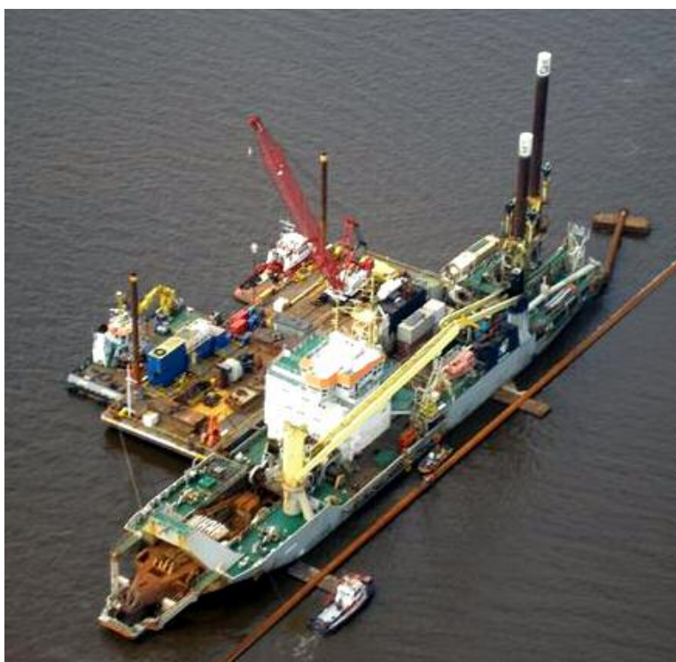
Top view of csd Ursa preparing a sinker pipeline at Soyo LNG project Angola with alongside the Barge Stemat 79 , BKM 103 and Ijsselstroom .
