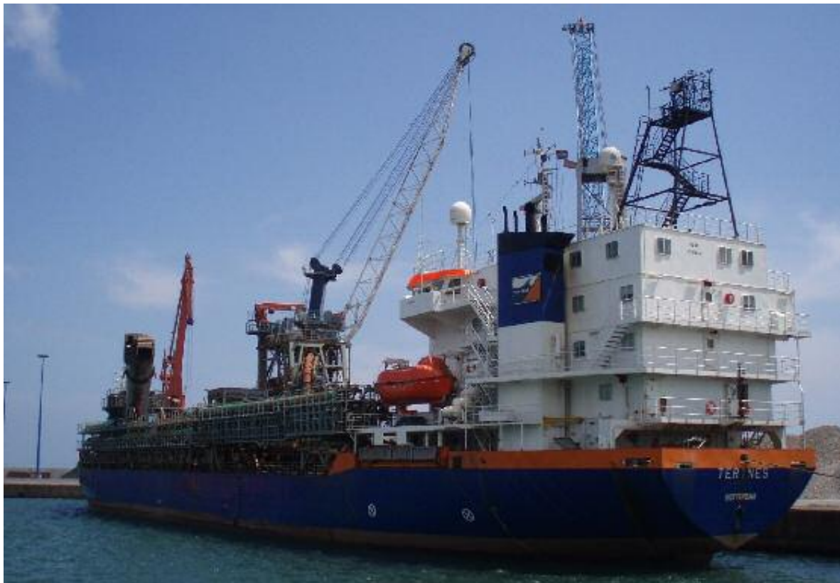
The flexible fallpipe vessel Tertnes , alongside in Gijón Spain working on the fundation of a new harbour breakwater.
