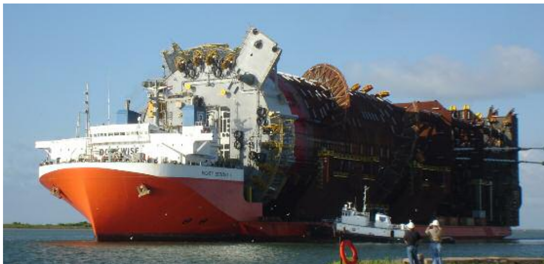
The MIGHTY SERVANT 1 loaded with the TAHATI hull seen arriving in Ingleside (Texas)
