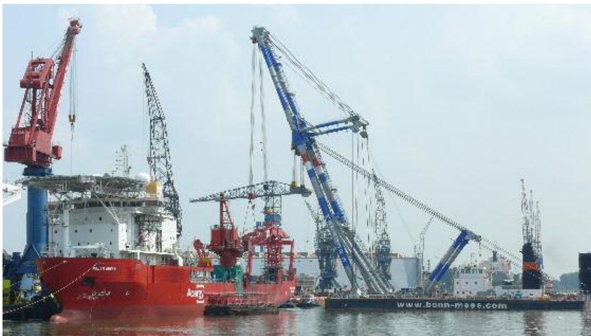
The sheerlegs MATADOR 3 seen lifting the crane boom onboard the POLAR QUEEN in Wilton Harbour (Schiedam)
