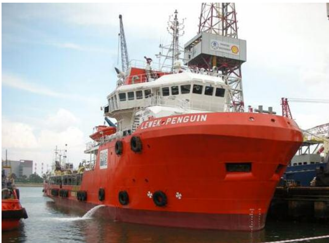
Lewek Penguin seen at Pan United shipyard in Singapore, just completed her seatrials Two x Rolls Rolls 5548 HP and 160 T Bollard Pull, full complement for 40 , DP-2
