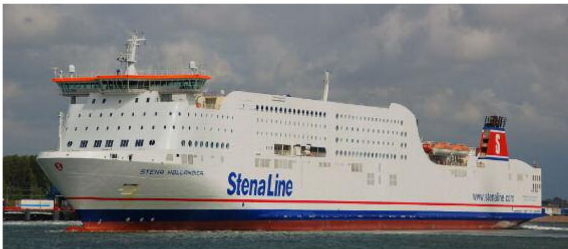
The 51.6 mtr lengthened STENA HOLLANDICA seen departing for the first time from Hoek van Holland, The 44.237 GRT STENA HOLLANDICA is now having a total length of 250 mtr.
